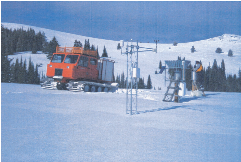
Plate 2. Climate, snow, and precipitation measurement site near Fir forest in the southern, higher-elevation region of the Reynolds Creek Experimental Watershed during December. Snowcat is used for instrument maintenance and data collection during winter.
